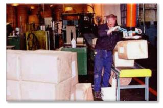
The example shown is palletizing using a vacuum lift at a paper mill that produces bundles of grocery bags.
