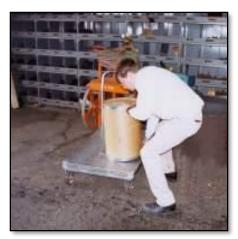
This is a relatively common device used in industry – a scissor-lift cart. The height of the cart is adjusted hydraulically, in this case with a foot pedal, although powered adjustment mechanisms are also available. These carts cost about \$1,500.
