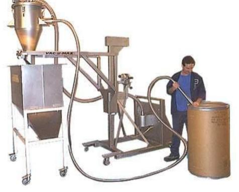
This example shows a mobile pneumatic conveyor that can be used to move powdered and granular materials from any type of container (bags, barrels, bins, totes, etc.) to a hopper or other part of a mixing system.
