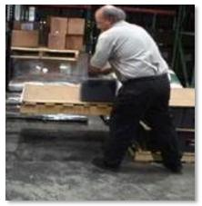
This example shows how to move heavy duty batteries from one pallet to another when picking an order.
